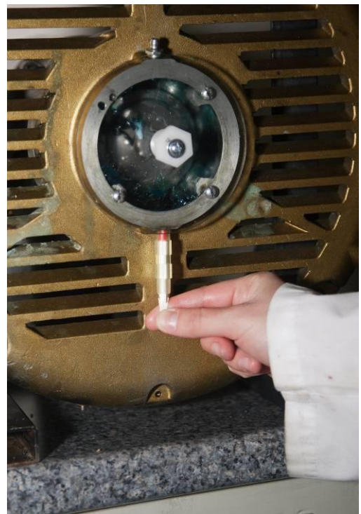
Figure 1: Grease sampler installed in a motor test stand
