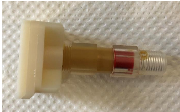
Figure 30 Filled Grease Thief without piston
