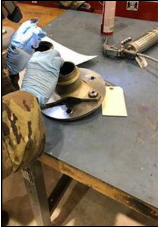
FIGURE 4: Soldier obtains spline grease sample during maintenance activity
