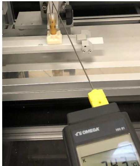
Figure 31 Omega thermocouple embedded in Grease Thief
