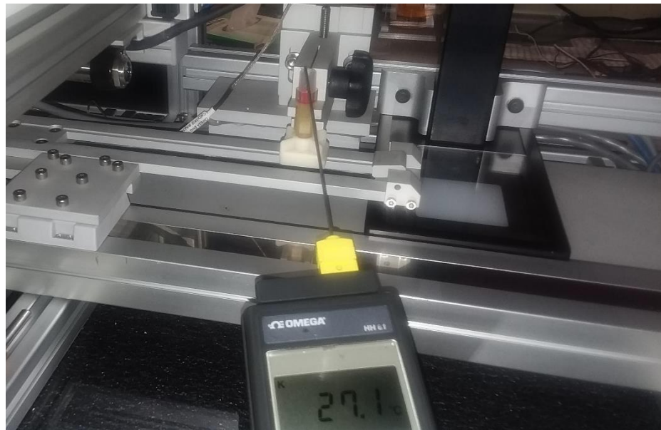
Figure 32 Thermocouple embedded in Grease Thief to test with IR sensor
